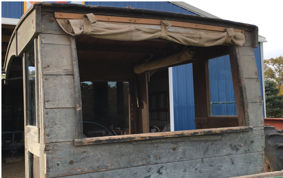
Instead of glass where normally is a rear window a canvas curtain rolls down to keep out rain
